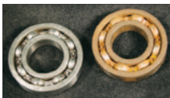
The bearing on the left was treated with CorrosionX; the one on the right was left untreated. Both were sprayed with seawater every day for two weeks. Note the remarkable difference.
